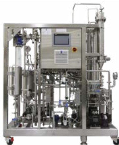
Flavourtech's SCC100-W has a throughput of 25-120 litres per hour and has been designed for use in a laboratory, pilot plant or for small production runs.
