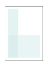
Third Page (TP) (no bleed) Horizontal - 90mm H x 185mm W Vertical - 272mm H x 59mm W
